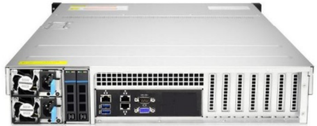
Rear View of 7-PCIe Rear Window
