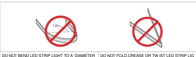
DO NOT BEND LED STRIP LIGHT TO A 'DIAMETER LESS THAN 1.5 INCHES.
