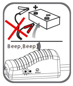
Green Light Blinking with Buzzing: The vehicle battery is low, press the "BOOST" button, wait for the Green Light stability, then start the engine within 30s.
