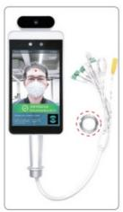
1. Unscrew the nut at the bottom of the gate head post, thread the cable out of the nut, and remove the nut.
