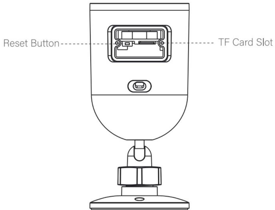
Please open the cover with a screwdriver to insert or remove a TF card. (The reset button is designed inside)
