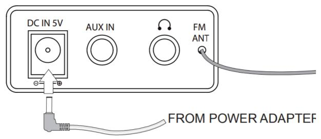
3. Plug the Power Adaptor in a mains outlet socket and switch on.
