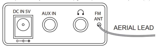
2. Plug the connector on the lead from the Power Adaptor into the DC IN connector on the rear panel.
