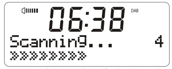
7. When scanning is complete, the first found station will be played. Press the < or > buttons to select a different station.
