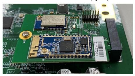
This Limited module is installed in the End-product for USB-C Smart Dock (M/N: DUD8070)
