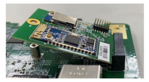
2. Secure the module to the motherboard with screw. (Figure 2)
