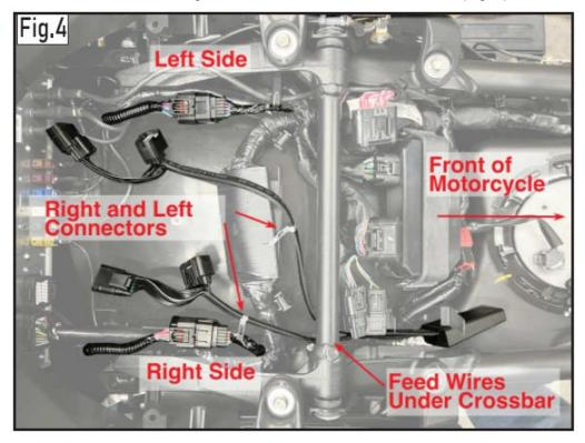
4. Determine left and right Goldstrike connector plugs by checking the labels, then plug them in-line with the factory wiring connectors you disconnected in step 2. The large connectors should be placed out of the way so the seat will not crush them. (Fig. 5)
