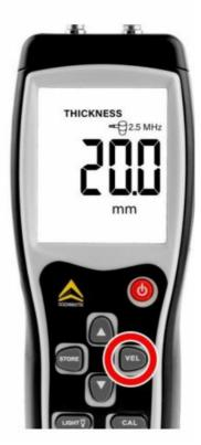
• As a last step, you press the VEL-button once again. The device then calculates the correct speed of sound. Having done this, you can scan the rest of the bar like you did in measurement 1.
