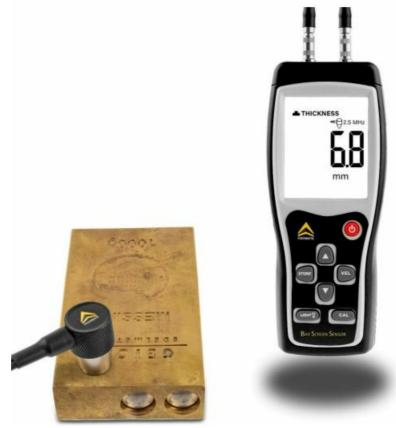
• Of course, this value is incorrect because the previously selected sound speed is wrong. This is why you now take off the measurement head from the bar and measure the objects thickness with calipers. Use the arrow keys to adjust the thickness for the BarScreenSensor in a way that it matches with the actual thickness.
