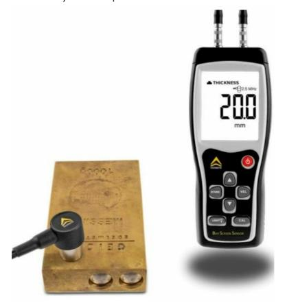
• After this, you should "scan" the bar. To do so, you lay the measurement head on different spots to exclude inclusions of foreign material. In case of a fake, the value of the thickness can differ significantly.
