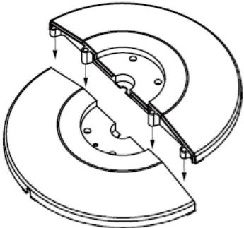
Position the base half with the alignment pin, over the other base half with the alignment sockets. Press the two halves together until flush. Assemble the base to the tower bottom. With the tower on its side, align the 4 base sockets onto the tower bottom pins. Tighten the screws securely but do not over tighten.
