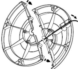
Assemble the two base halves together.
