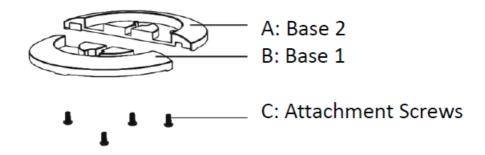
Lock base in place with 4 screws supplied (C).
