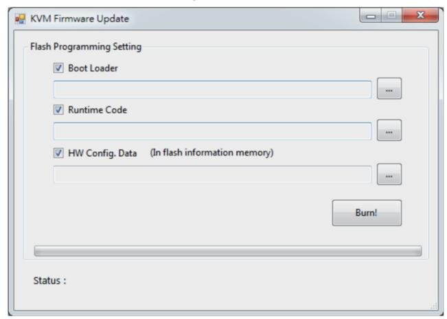
5. After updating, please set the dip switch PIN#1 to OFF [†] and power cycle the device
