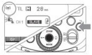
Press < \*\*- > button so that < (\*\*) > or < SLAVE > are displayed on the LCD panel.
