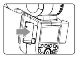
2. According to the triangle sign on the battery pack, insert it into the compartment until a white knob locks the battery with a click sound.
