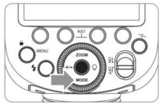
2. Press the <+/-> button and turn the Select Dial to choose a desired flash output amount.
