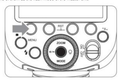
2. Press <MODE> button to switch to Multimode.
