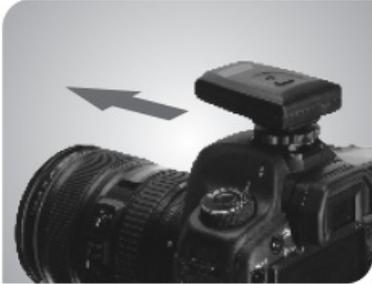
4. If the camera has no Hot Shoe Jack, insert one end of the synchronous line into the Socket for Synchronous Line (8) and the other end into the Synchronous jack of the camera.
