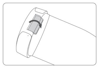
Press down the fixing pushers on the both sides, insert the adapter holder into the projection attachment then let go the pushers.
