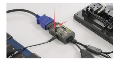
Step 6: Press the start button and the red ignition switch button again.
