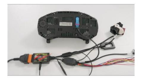
**Step 1:** Connect GT115 to the instrument panel and power it on.
