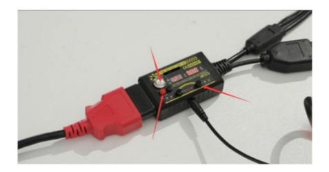
**Step 3**: Press in sequence: power switch start, ignition switch IGN, engine button switch ENG.
