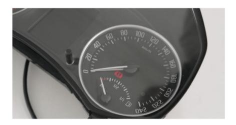
**Step 6**: At this time, only one light is on, indicating that the instrument has successfully entered the pogo pin mode.
