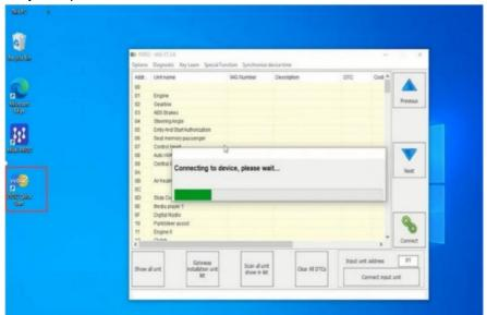
**Step 3:** Select"VW">>"K-Line Instrument/Immobox">>"Instrument Cluster(VDO66, VD086, Motometer)">>"Read EEPROM">>"Save File".
