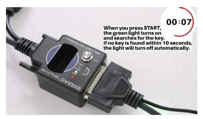
**Note:** When you press the START button, the green light turns on and searches for the key. If no key is found within 10 seconds, the green light will turn off automatically.
