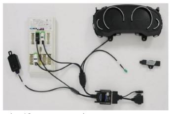
2. Step 2: Then connect the 12v power supply.
