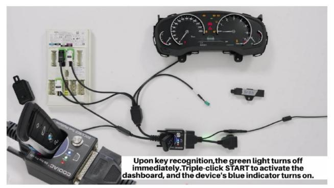
5. **Step 5:** Press the START button two times in succession. Please note that the interval is about 0.1S. Alternatively, you can also press and hold the START button to turn off the blue IMMO light and dashboard.
