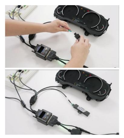
2. **Step 2**: Press the START button and put the key in the sensing area, the green light will go out immediately indicating that the key and the BDC3 module are synchronized.
