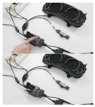
3. **Step 3**: After we took away the key, the green light did not light up, which means that the key has been recognized.
