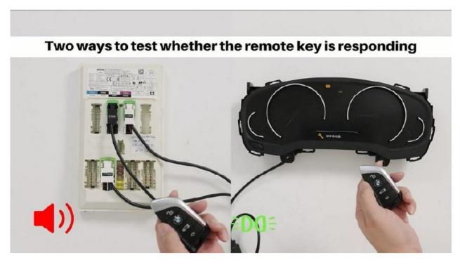
3. **Step 3:** After pressing the unlock button on the key, the remote control receiving module makes a clicking sound and the green light on the dashboard lights up. Either of these two methods can test whether the remote control key responds.
