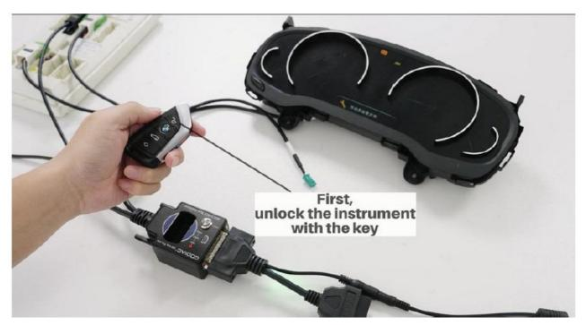
2. **Step 2**: Press the START button once, the green light will come on, and if the key cannot be found within 10 seconds, it will automatically go out.
