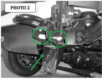
• Step-1: Remove the bolts (3) per side securing the tow hooks and bumper bracket assembly to the frame,
