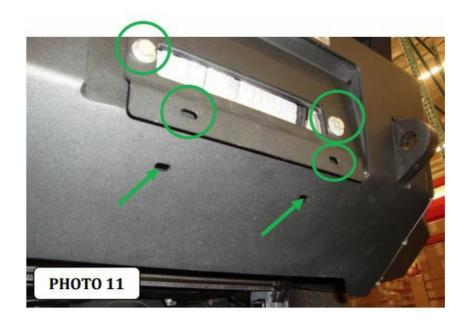
If your state law requires a front license plate, attach the license plate bracket to the holes in the face of the bumper shell, using the supplied 3/8" bolts, washers and nuts, and the license plate to the (2) obround holes in the license plate bracket using the supplied 1/4" bolts and nuts. (Photo 11).
