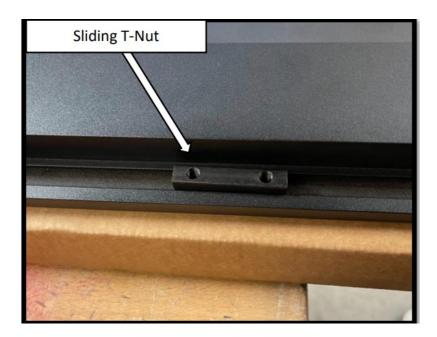
**Step 9**: Determine where you want to position the board and secure the running board to the arms using the (2 per bracket) M6x25 socket head cap screws. Using a torque wrench, tighten to 9 ft-lbs. Step # With the running board is installed, fasten the hardware on the Driver side front and rear motor assemblies. Using a torque wrench, tighten the mounting hardware to 18 ft-lbs.
