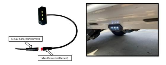
**Step 13:** Align the arrows on the small round connectors and plug the Passenger side front and Passenger side rear LED lights. Prepare the surface by cleaning with a 50/50 mix of isopropyl alcohol and water or equivalent. Once the surface is completely dry, peel the backing from the double-sided tape and stick the LEDs to the bottom side of the rocker panel. Position the LED lights at the center of the front and rear passenger side doors
