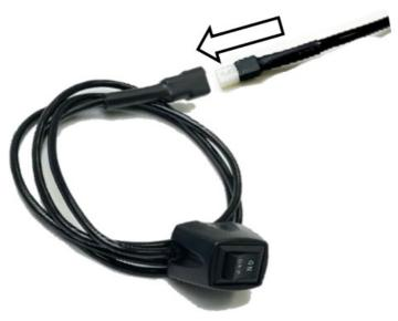
**Step 24**: Remove the 20 Amp fuses from the main positive and negative 12V power leads on the main harness. Route the power wires over the wheel well and into the engine compartment. Connect the ring terminals to the battery positive and negative terminals. Install the 20 Amp fuses back into the main negative and positive power lead fuse holders. Connect the battery terminals. Begin with the positive terminal followed by the negative terminal.
