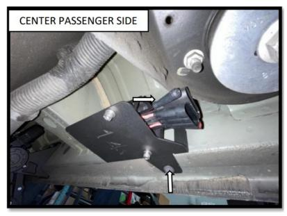
**Step 8:** Install the Passenger side running board. With assistance, begin by positioning the board on the front and rear motor assembly bases. Align the sliding T-Nut on the running board with the slots on the front and rear motor base. Once the T-Nuts are aligned, rotate the running board so that the T-Nuts set in the slots on the base of the arms. Repeat Steps 3-6 to install the motor linkage assemblies and running board on the Passenger side.
