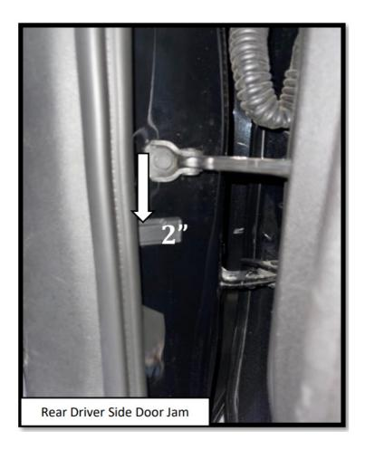
**Step 21:** With the rear driver side sensor attached, you can determine the correct position for the door magnet. peel the backing from the double-sided tape and stick the magnet on the door. Align the bottom of the magnet with the 4 1/2"
