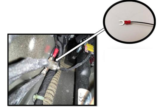
Connect the snap-in bullet connector to the brown wire on the Passenger side b-pillar
