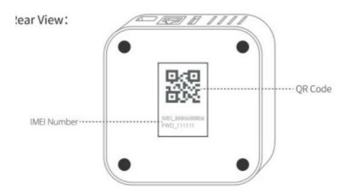
Scan the OR code containing IMEI number on the back of SIMBOX to bind device. And you can also input IMEI number and password to bind device. See the figure as above.
