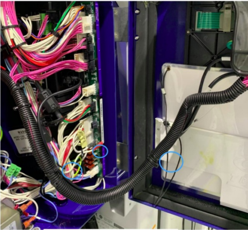
Figure 7a: Securing wire harness
