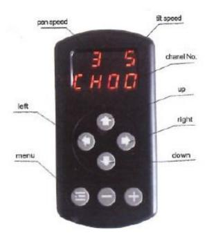
The remote control is powered by 2AAA alkaline battery, when the battery is installed, press any key to activate it, after stopping,..operation for 8 seconds the remote control will power off. Press the left and right key, the pan operates, press the up and down key, the tilt operates. Press the menu key, can adjust the pan and tilt speed.
