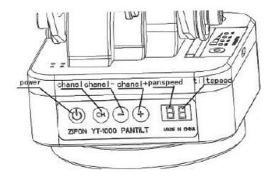
Power on, the led display on Press the CH, will indicate the Chanel No., the Chanel No. is between 00-19 \ w, Press- or+ to change the Chanel No., the Chanel No. on the pan tilt must be same as the Chanel No. on remote control. The display indicates pan speed and tilt speed, the speed adjustment should be made on remote control.
