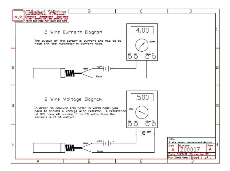
Appendix B: 2 Wire Sensor Measurement Diagram
