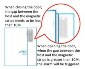
Please note during installation: the triangle mark on the side of the host must be aligned with the mark on the magnetic stripe.
