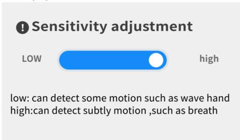
**Tips**: If the detected object is in a range of 3 meters, even a low sensitivity had been set, the micromovement also can be detected.
