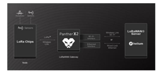
Panther X2 sends and receives LoRa data, modulates/demodulates signals, processes LoRa data and higher-level protocol-related tasks, and eventually transmits data to the server via Ethernet or Wi-Fi.
