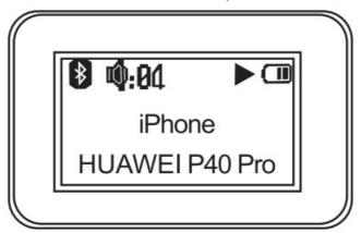
**Note:** The default play source is the first connected device. If you want to switch the playback device, please hit pause on the current device, then hit play on the other device.
