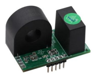
The IM1281B single-phase AC electricity metering module is developed in order to adapt to various manufacturers to monitor the power consumption of their products; it is also an suitable module for AC charging pile, street lamp, computer room, base station to save energy and monitor. The accuracy is better than the national level 1 standard;
