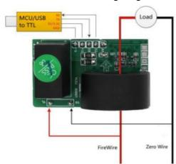
IM1281B Schematic diagram of pulse detection interface wiring Pulse Output detection Circuit
