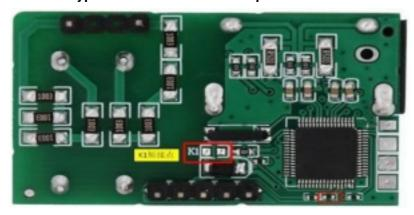
If the connection is correct, the communication indicator flashes, but the data does not return, please short-circuit this current-limiting resistor and then communicate.
