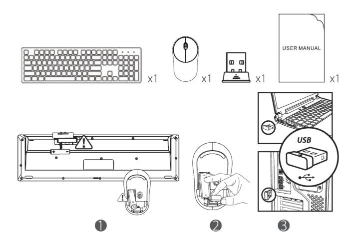
Remove the battery cover under keyboard and insert one AAA battery. Plug the receiver into the USB port of computer. Please wait for about 3s and the drive will install automatically for your usage.
