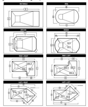
• Be sure that the length (A) and the width (B) measurements are made at the pool wall, NOT at the edge of the coping (the edge of the pool deck). The pool coping usually extends beyond the pool wall and will give you an incorrect length and width measurement. See illustration below.
