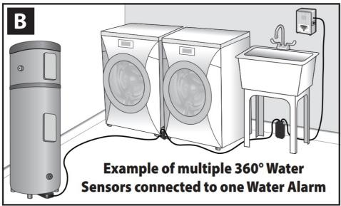
This will allow you to monitor multiple locations for water damage. First remove the rubber plug from the 3.5 mm jack and then plug in additional sensors.
