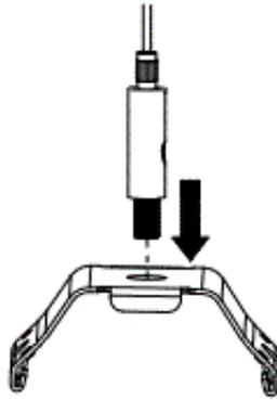
2c Lock coupling apparatus on the metal dome without.
