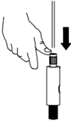
2b Insert the coupling apparatus with sling through hole dia 10mm on the metal dome.
