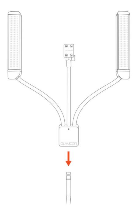
05. secure the luminary by tightening the knob
