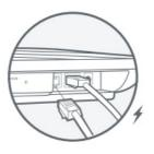
Plug the cable connecting to your computer into LAN port
