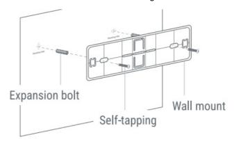
2. Connect the router to a power supply and insert an ethernet cable, then attach the router to the wall mount.
