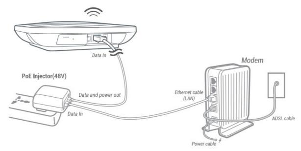
! This router does NOT work with 24V PoE injectors.
