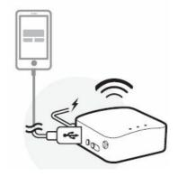
Using the USB cable to share the network from your smartphone or hostless modem to the mini router is called Tethering.
