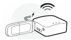
Plug your 3G/4G modem into the USB 2.0 port of the router, and it can transfer the 3G/4G signal to Wi-Fi.
