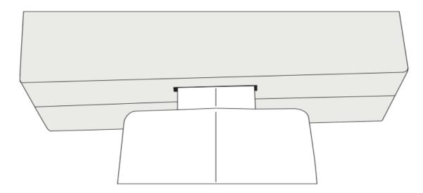
2. Align the mounting frame, mark the drilling holes, drill and insert wall plugs.
