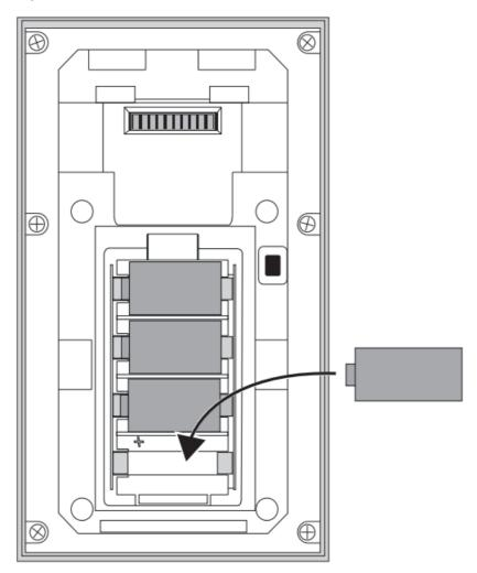
3. Attach the wireless control unit to the mounting frame (attach from above and swivel in from below).
