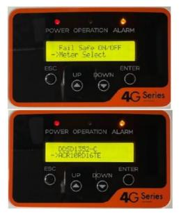
**STEP 11:** Now turn the Grid ON in Advanced Settings. (Go to Advanced Settings again by pressing ESC thrice < Set password 0010 < Go to Grid ON/Grid OFF < Select Grid ON < Press Enter).
