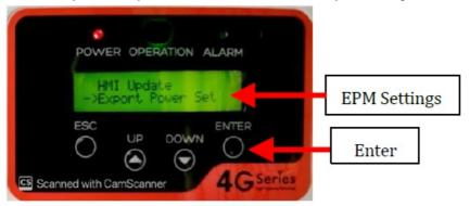
**STEP 6:** Use Up/Down keys to scroll to EPM settings/ Internal EPM/ Export Power Set, whichever is available on your screen. Then press Enter.
