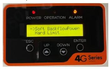
**Step 8:** Choose Soft Backflow Power and press Enter. Then set the export limit using the Up/Down keys and press Enter to save. For example: 5kw export limit will be +5000 W.
