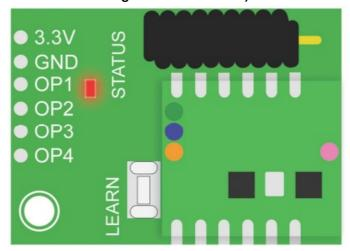
• To pair a compatible remote, briefly press the small white program/learn button (see illustration to the right), the Red LED should illuminate while you press and then after you release (~1s later) it will flash once to indicate that the receiver is ready to pair to OP1. To program OP2, briefly press again, and afterward, the LED will flash twice, for OP3 press a third time and wait for 3 flashes, or for OP4 a fourth time and then it should flash 4 times.
