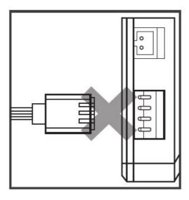
Do not connect the 3-Pin ARGB to the 4-Pin RGB heater of the motherboard, which will damage the fan lighting. If your motherboard has no RGB function, you do not need to connect the 3-Pin ARGB
