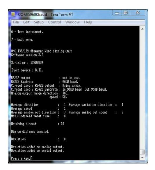
To change the input device from an anemometer configured for Gill output mode, 9600 Baud to a device configured for NMEA mode, 4800 Baud, follow the steps below:
