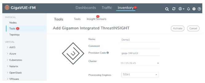
GigaVUE-FM creates the required configurations, such as the GigaSMART group and the Virtual port on the SMT-HC1-S module. GigaVUE-FM, then establishes connection with the ThreatINSIGHT Sensor using the provision code you provided. The ThreatINSIGHT Sensor communicates with the Gigamon ThreatINSIGHT Portal and
