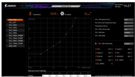
Use the <F6> function key to quickly switch to this screen. This screen allows you to configure fan speed related settings for each fan header or monitor your system/CPU temperature.
