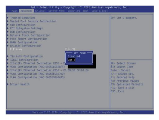
5. When ErP Mode is enabled, fan speed will be adjusted and any redundant PSU will be placed into a standby state ("Cold Redundancy") in order to decrease power consumption when the server is in idle mode.
