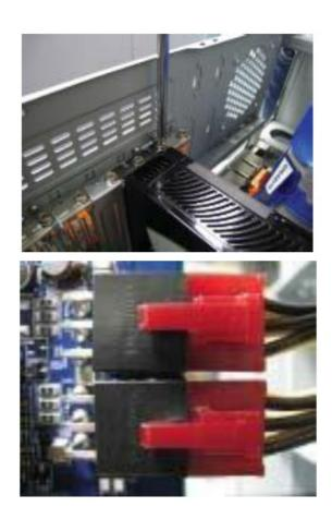
If there are power connectors on your card, remember to connect the power cable to them, or the system will not boot. Do not touch the card when it's operating to prevent system instability.
