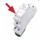
• After holding the switch for 5 seconds, if the LED light is red, press the switch again and you will see the green light blink
