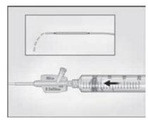
11. Prepare a 20 cc syringe or balloon inflation device with saline or diluted contrast mixture and attach to the balloon inflation port (labeled I on the catheter hub). Hold the delivery system vertical with the distal tip pointing
