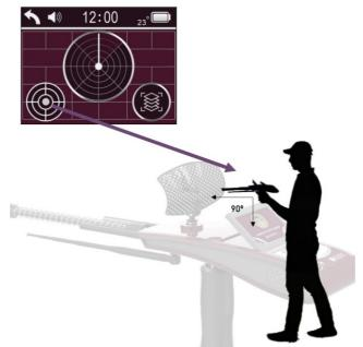
The balance of the device must be maintained during the search by fixing the grey dot in the middle of the circle icon.
