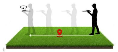
Follow the signal and when the device turns back you will have passed the target.
