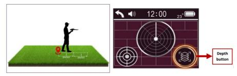
After you have confirmed the location of the target, click on the depth button to determine the depth and then move away from the center of the target a distance of at least 2 meters.
